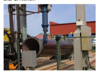
There were tested the large-sized structures (structural beam and section of the typical vertical column) from nano-modified composite materials on the base of the domestic polymer resin and continuous glass reinforcement filler (the development of VIAM). The tests were conducted on the unique equipment located on the reinforced floor of GCCT.
